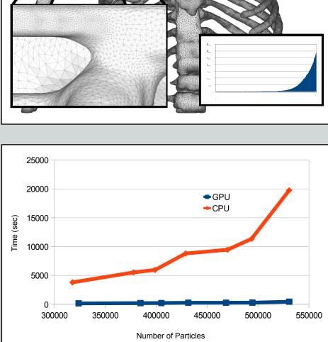
Timing results, in seconds, as the number of particles increase. The GPU times are in blue while the CPU times are in red.
