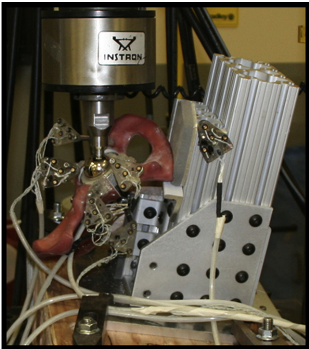
Fig. 4. Photograph of custom Instron mounting jig attaching the hemipelvis through the sacroiliac and pubic-symphyseal joints via semideformable spacers.
