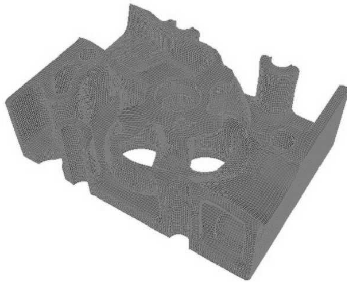
Figure 6.31. Hexahedral mesh of the test1 model.
