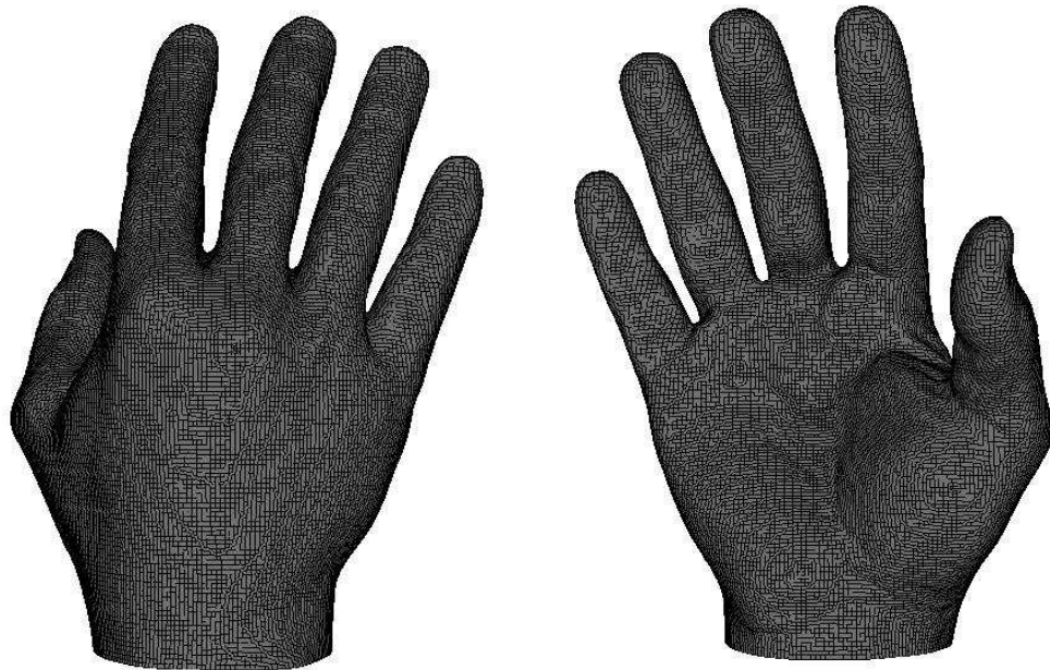
Figure 5.20. Front and back view of the hexahedral mesh of the hand. The mesh contains 202,974 elements.
