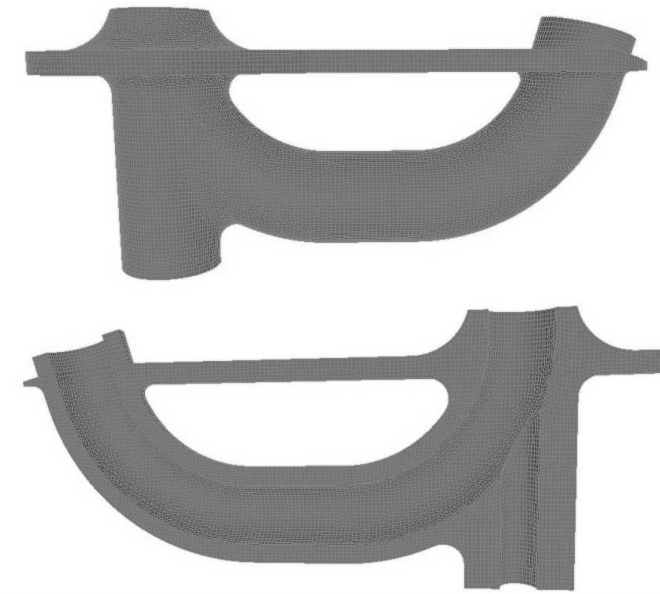
Figure 6.28. Hexahedral mesh of the goose16 model showing images from the front and back of the mesh, respectively.
