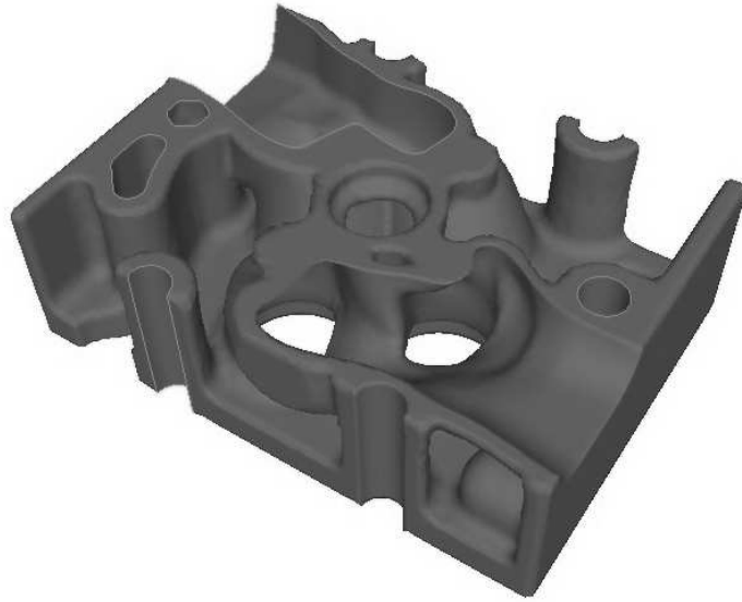
Figure 6.34. Image of the geometry generated from the hexahedral mesh of the test1 model.
