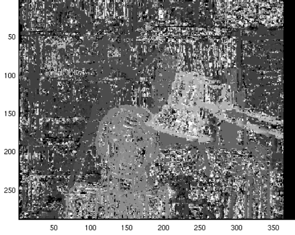
Figure 10: Disparity map associated to the previous rectified stereo pair
