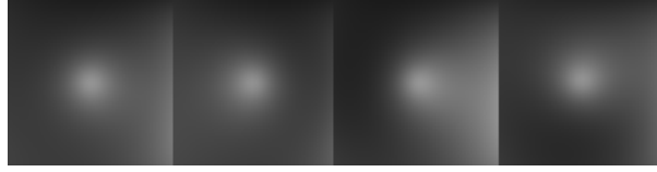
Figure 15: Four images with different light source position used to reconstruct shape
