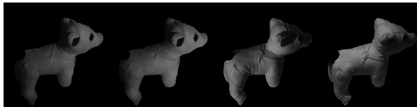
Figure 31: Four dog images with different light source position used to reconstruct shape
