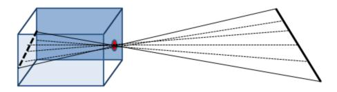
**b**) Show that, in the pinhole camera model, three collinear points in 3-D space are imaged into three collinear points on the image plane.
