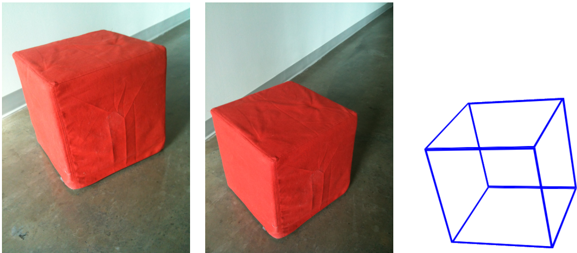
Figure 3: Two pictures of a simple geometric object (here vertical stereo) and its 3D reconstruction with a wireframe illustration.
