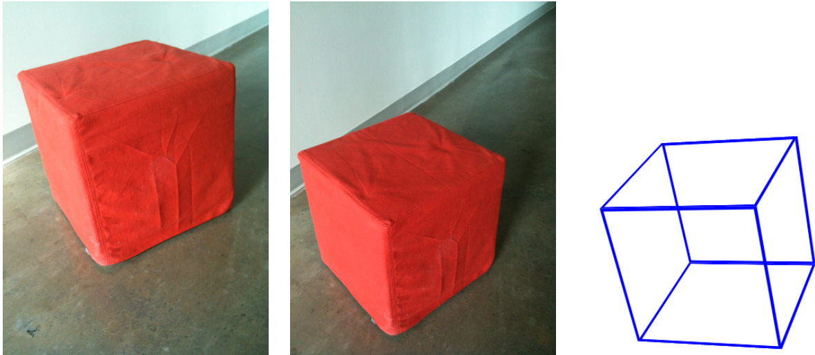
Figure 3: Two pictures of a simple geometric object (here vertical stereo) and its 3D reconstruction with a wireframe illustration.
