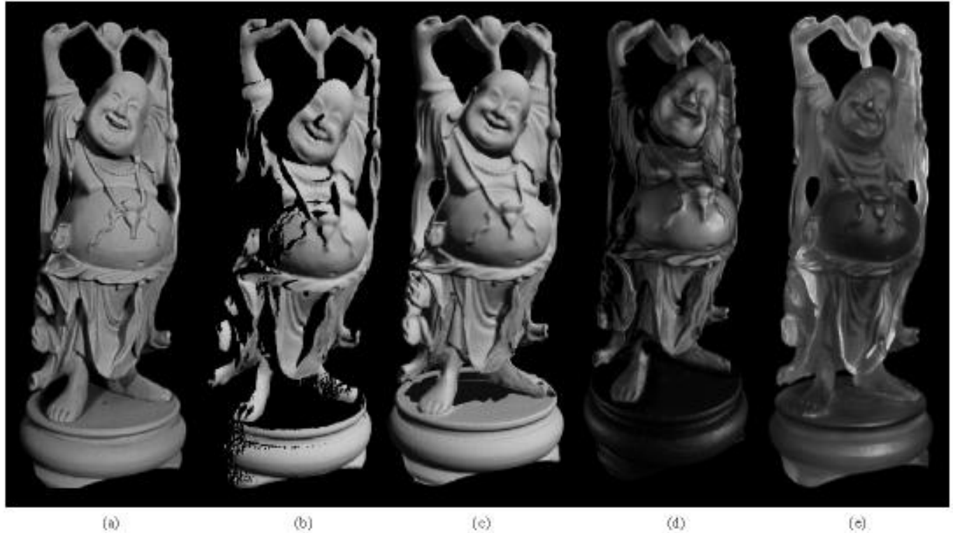
Figure 24.17. 3D Fax of a statuette of a Buddha. From left to right: photograph of the statuette; range image; integrated 3D model; model after hole filling; physical model obtained via stereolithography. Reprinted from [Curless and Levoy, 1996], Figure 10.
