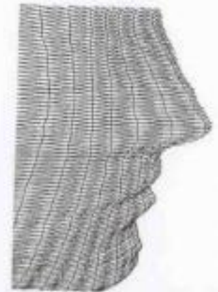
Figure 9.10: Left: Rear view of the recovered 3D profiles of the Beethoven statue shown on the left of Fig. 9.9, Right: Recovered triangular mesh around nose and mouth of the statue.
