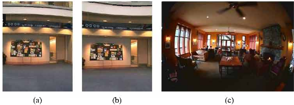
Figure 2.13 Radial lens distortions: (a) barrel, (b) pincushion, and (c) fisheye. The fisheye image spans almost 180^\circ from side-to-side.
