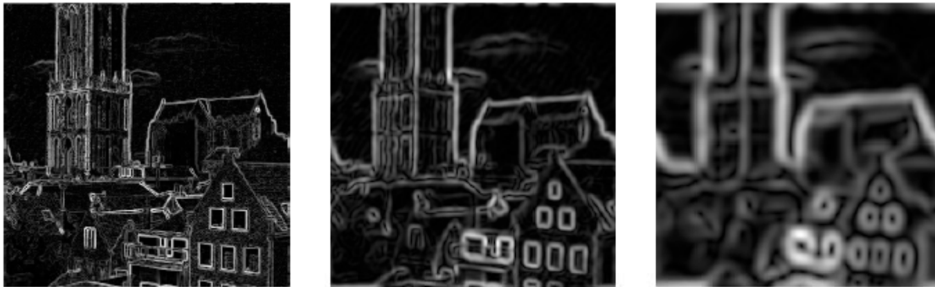
Figure 5.11 Gradient edges detected at different scales ( \sigma = 0.5, 2, 5 pixels resp.). coarser edges (right) indicate hierarchically more 'important' edges.
