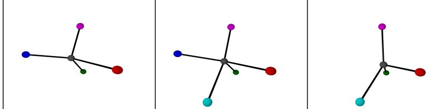
Lithium (gray) gains a bond with cyan oxygen, creating an unstable configuration, causing it to shed the blue oxygen. Plots of topological properties help understand reconnection events.
