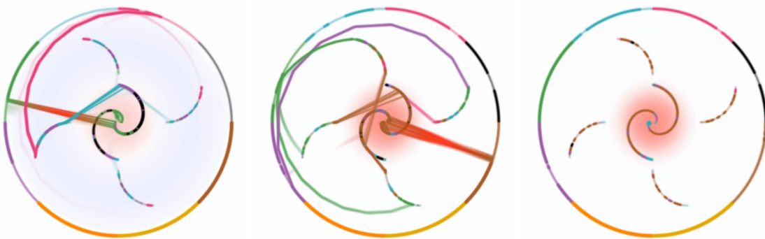
Figure 5.4. Visualizing the material point method in Waxlamp. The material point method (MPM) is a particle-based mechanical engineering simulation method. Left: Computation of momentum from the mass and velocity data (in the black and green arrays). The algorithm tends to sweep through the values in order, resulting in good cache performance. Middle: Computation of the particle stress update (brown data array) near the end of the timestep, from various data, including the constitutive model (blue data array). MPM is made up of several phases which tend to access the data in order. The resulting visual pattern is that of data moving into L1, being operated upon a limited number of times, and then slowly migrating first to L2 and then back into main memory, as newer data comes into L1 to be operated upon in turn. Right: This example shows a bigger MPM simulation and a larger cache to demonstrate Waxlamp's scalability.
