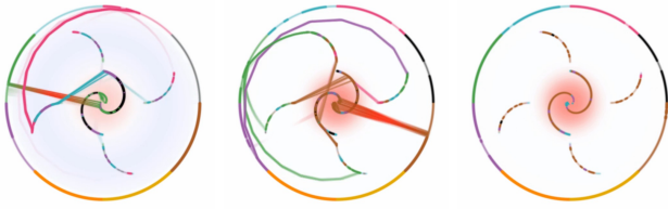
Fig. 8. The material point method (MPM), a particle-based mechanical engineering simulation, in action. Left: Computation of momentum from the mass and velocity data (in the black and green arrays). The algorithm tends to sweep through the values in order, resulting in good cache performance. Middle: Computation of the particle stress update (brown data array) near the end of the timestep, from various data, including the constitutive model (blue data array). MPM is made up of several phases which tend to access the data in order. The resulting visual pattern is that of data moving into L1, being operated upon a limited number of times, and then slowly migrating first to L2 and then back into main memory, as newer data comes into L1 to be operated upon in turn. Right: This example shows a bigger MPM simulation and a larger cache to demonstrate the scalability of our visualization system.
