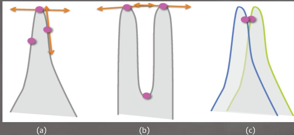
Fig: Incorrect correspondences near sharp features when (a) points with different tangent spaces interact, (b) nearby points sampling different parts of the surface interact, (c) optimization is based only on point positions on different shapes
