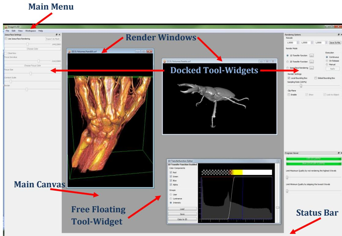
Figure 6 ImageVis3D's UI elements
