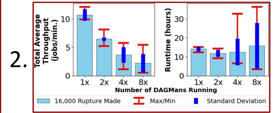
This figure illustrates the average total throughput and runtime of DAGMan workflows that ran parallel to create 16,000 ruptures using the full Chilean input.
