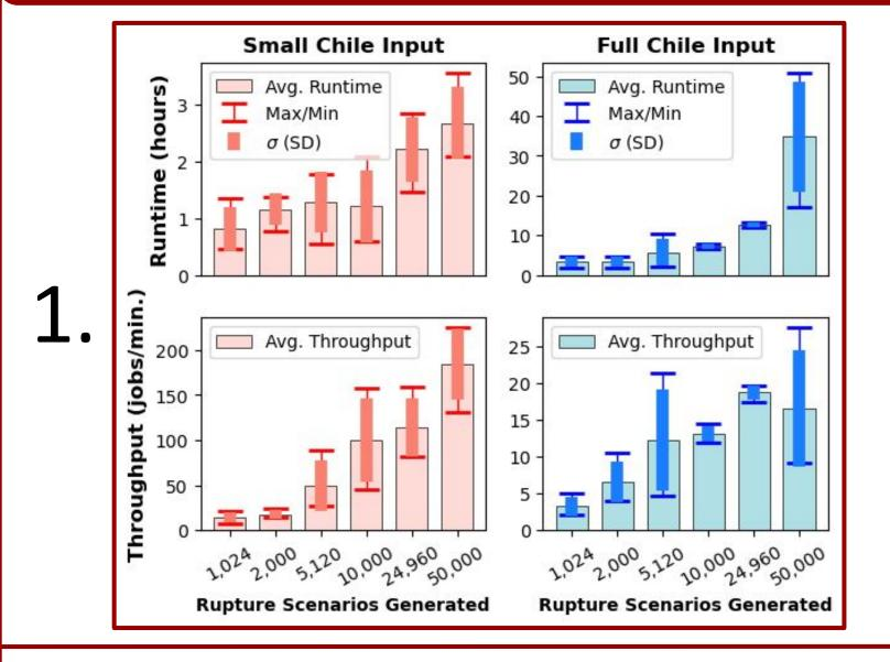
These graphs illustrate the average total runtime and throughput of the FDW simulating varying amounts of earthquake scenarios using two different-sized input lists (2 and 121 stations).
