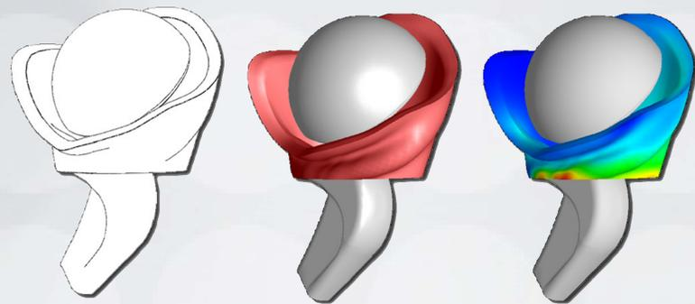
Figure 1. Finite element analysis of a hip implant device showing high stresses in areas of impingement.
