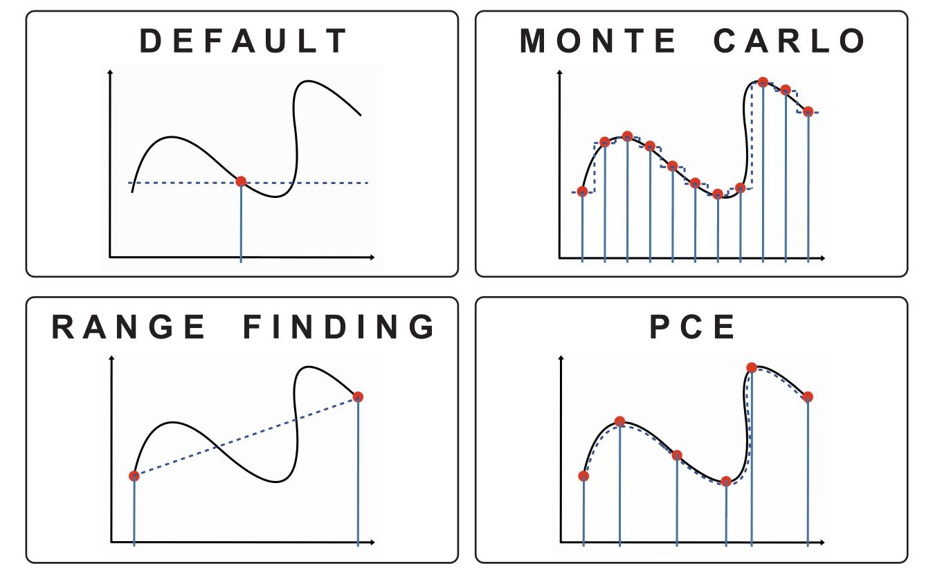
Polynomial chaos expansion (PCE) allows the user to effectively capture the parameter space with minimal computational cost. Members at the SCI Institute developed UncertainSCI which implements PCE via Python.
