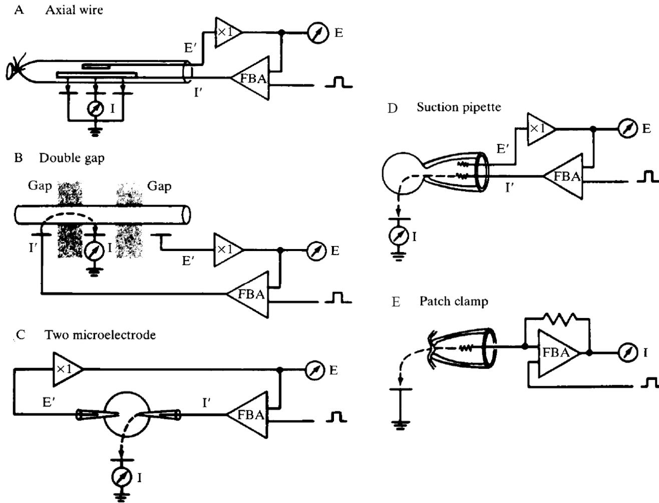
Fig. 3. Voltage clamp techniques. In each case FBA is the feedback (or clamping) amplifier,  $E'$  is the voltage electrode and  $I'$  is the current electrode. (Reproduced with permission from Hille, 1984).
