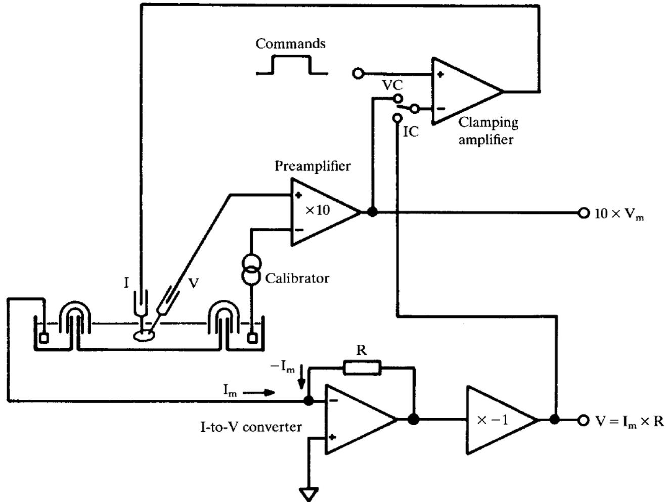
Fig. 4. Two electrode voltage clamp circuit. The circuit may be switched either to clamp voltage (VC) or current (IC).
