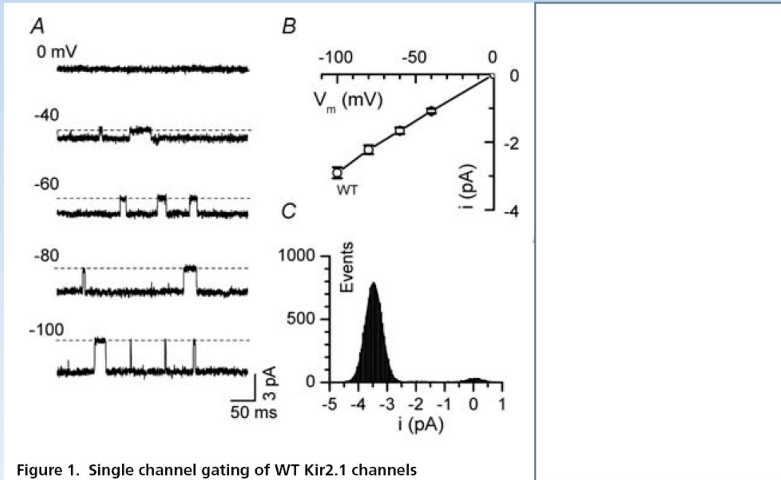
Figure 1. Single channel gating of WT Kir2.1 channels
