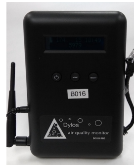
(a) Modified Dylos air quality sensor
