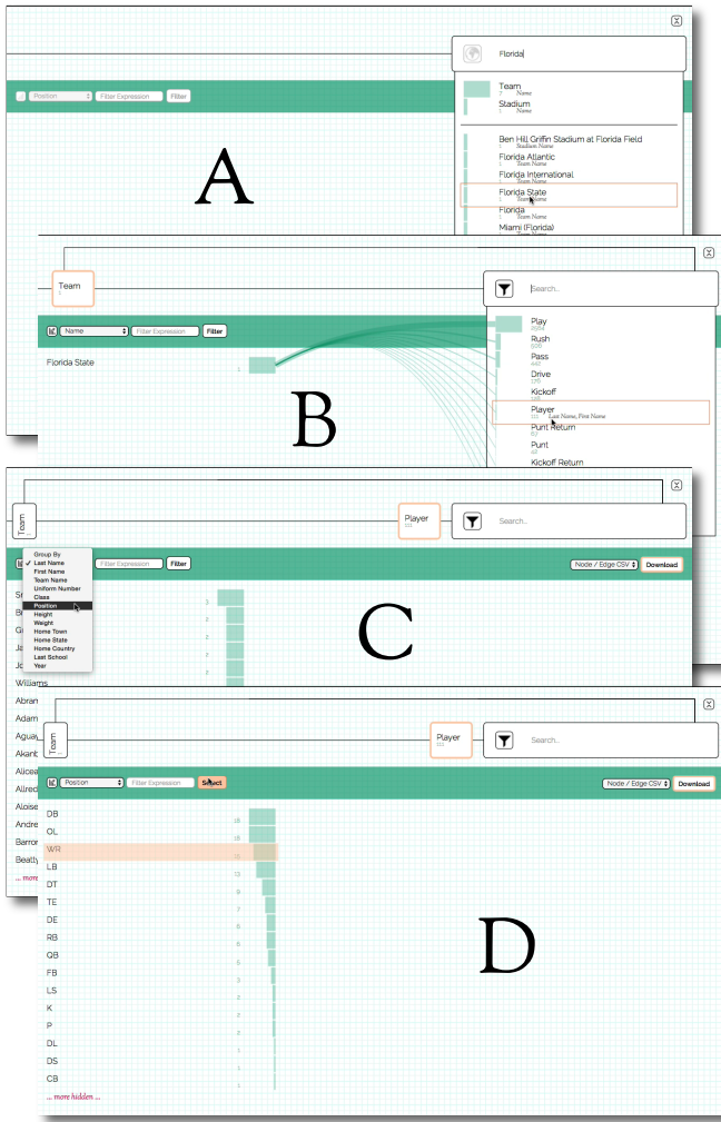
Fig. 3. Jacob's Ladder allows users to pivot from one category of nodes to another. A search box (A) shows search matches in the menu below. Matching nodes can be selected in aggregate, based on node type ("Team" or "Stadium" above the line), or individually based on value (below the line). Once a set of nodes has been selected, it is displayed as a histogram on the left of the search field (B). Subsequent searches are limited to the set of nodes that are connected to the previous selection, with line thickness encoding potential connections. The histogram supports regrouping and sorting (C), as well as selecting and filtering nodes (D) based on node attributes. The series of actions depicted are as follows: A) Florida State is selected, B) the user pivots to Florida State's players, C) players are grouped by position, and D) the wide receivers ("WR") are selected.
