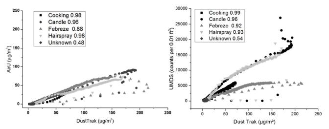
**Fig. 2.** Scatter plots and coefficients of determination ( $R^2$ ) of the linear model (low-cost sensor and DustTrak) for 5-minute rolling average of PM<sub>2.5</sub> concentrations ( $\mu$ g m<sup>-3</sup>) for several types of aerosols measured with a DustTrak (uncorrected), average of 4 AirUs (uncorrected) and average of 10 UMDSs, uncorrected (PM<sub>2.5</sub> count, small minus large bins, per 0.01 ft<sup>3</sup>) during 20<sup>th</sup>-25<sup>th</sup> May 2016 (Home I).
