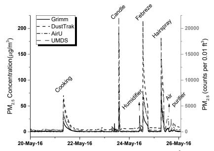
**Fig. 1.** Comparison of co-located 5-minute rolling average of  $PM_{2.5}$  concentrations ( $\mu g m^{-3}$ ) measured by a Grimm, DustTrak, average of 4 AirUs and average of 10 UMDSs ( $PM_{2.5}$  count, small minus large bins, per 0.01 ft<sup>3</sup>) for the calibration period of 20<sup>th</sup>-25<sup>th</sup> May 2016 (Home I). The concentrations measured by all sensors were uncorrected raw data.
