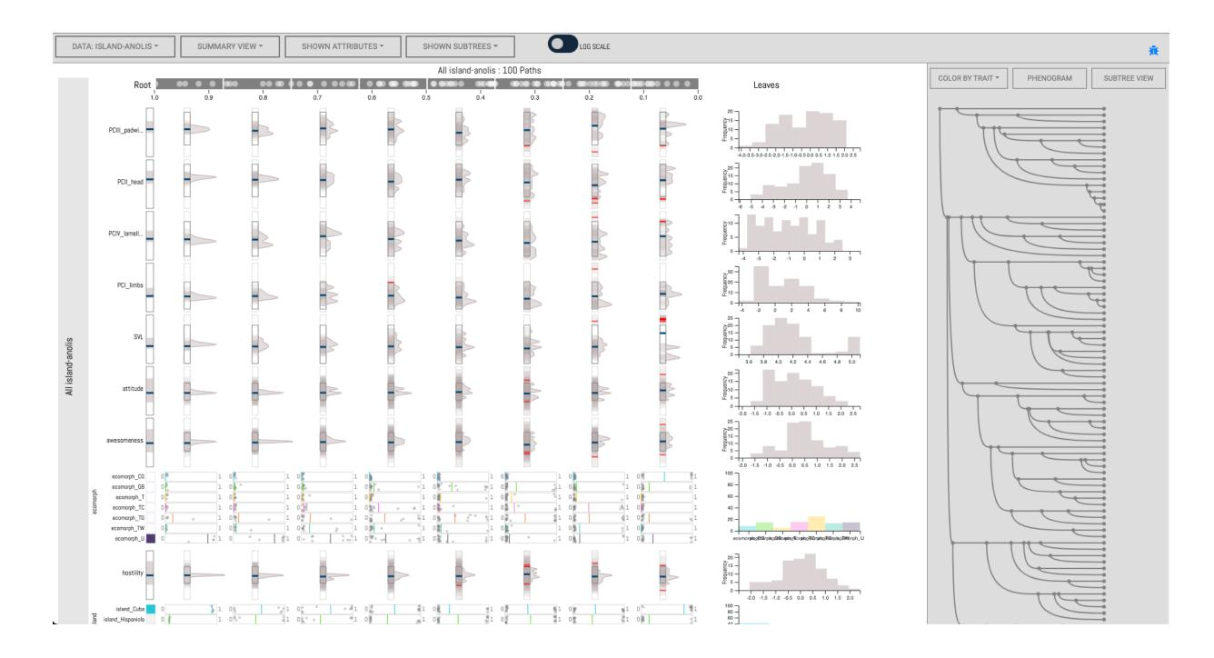
MultiLink: flexible node link diagrams layer out by topology or attributes. Attributes are also encoded on nodes & edges.
