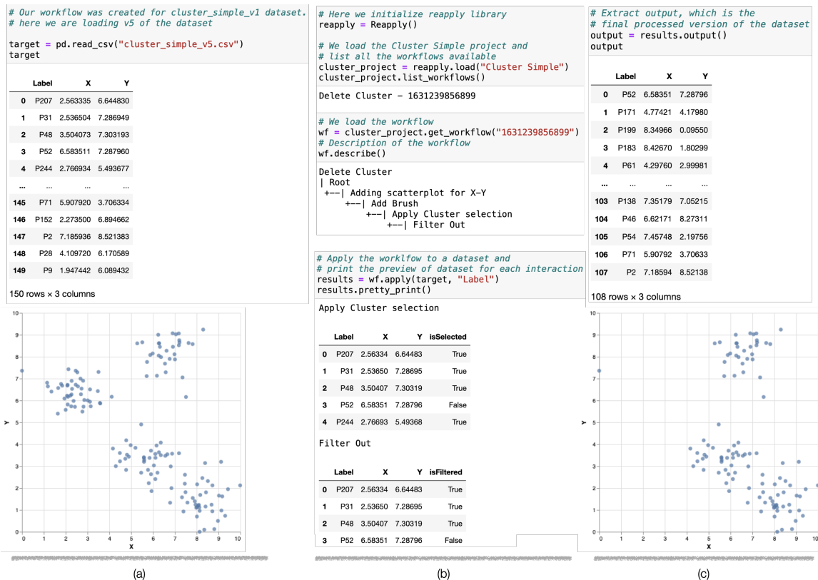
Figure 5.7: Executing a computational workflow defined in the visualization tool in a computational environment. (a) We first load the dataset. (b) We load the workflow library and the workflow we are interested in. We then apply the workflow to the dataset. The tool plots a preview of the actions. Note that new isSelected and isFiltered Boolean columns are introduced when a brush and Filter are added in the preview. (c) After the Filter is applied, the number of rows is reduced from 150 to 108. A visualization of the result shows the cluster was removed. Visit the notebook .
